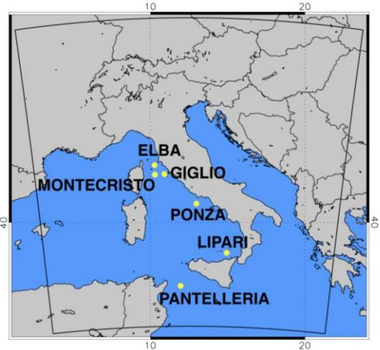
WRF model domain. The horizontal grid spacing is 3km. The yellow dots represent the islands' positions.
